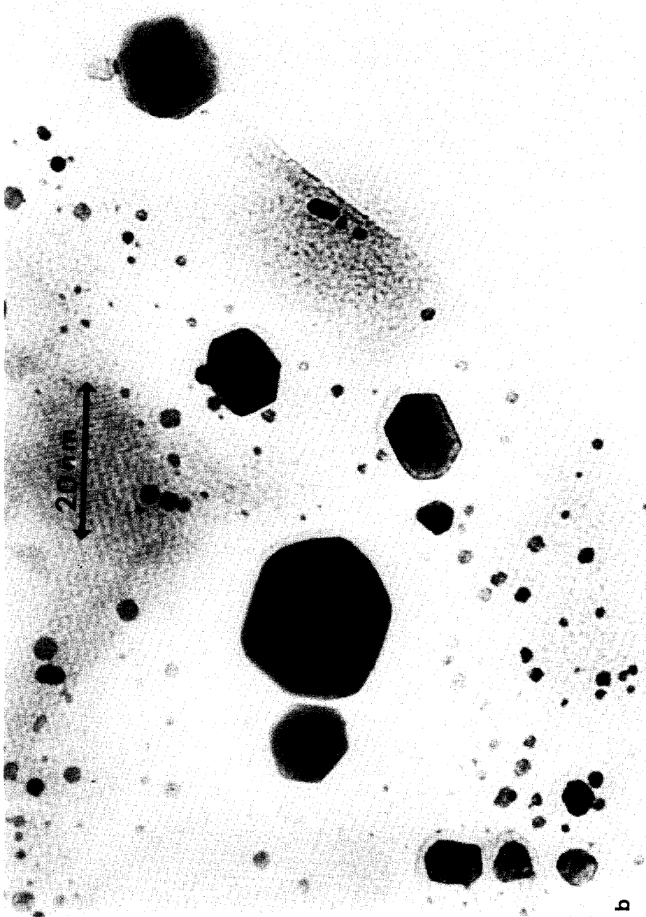
FIG. 1. Bright field images of Pt-Ni catalyst at different compositions (see the text for notation). (a) GNP100, (b) GNP75, and (c) GNP15.
