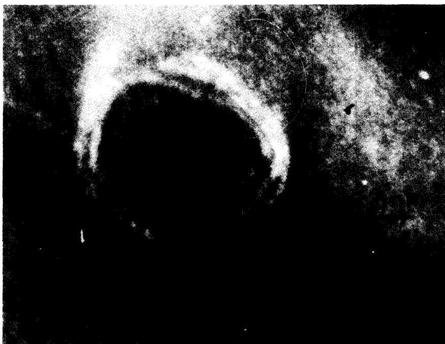
FIG. 2. Weak beam thickness fringes for a hexagonal particle which shows that the shape corresponds to a truncated cubo-octahedron.
